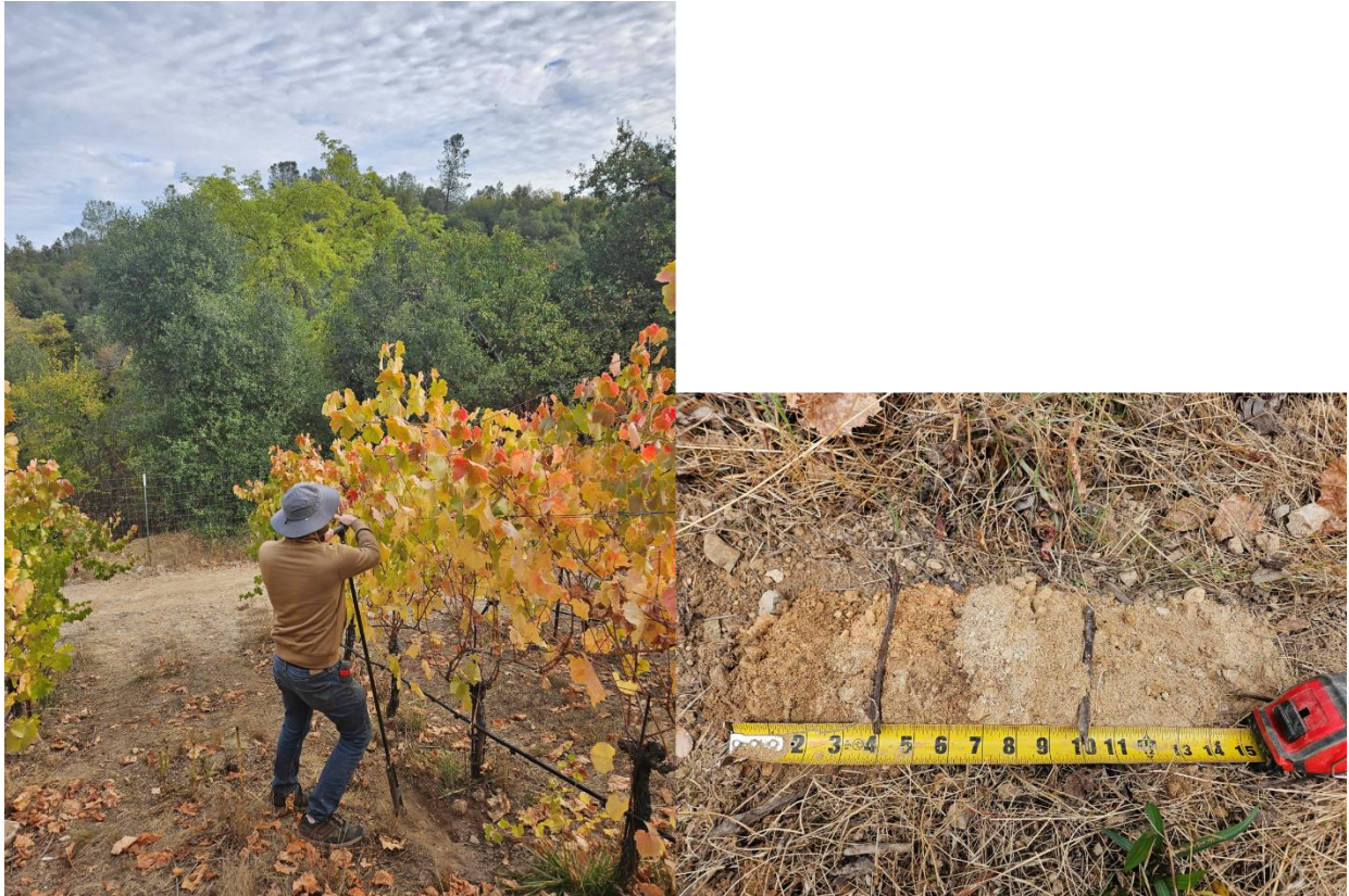
Figure 13. Field soil sampling process. The left panel shows a DE team member using an auger to collect one soil sample in a field. The right panel shows the resulting soil sample separated based on depth.
