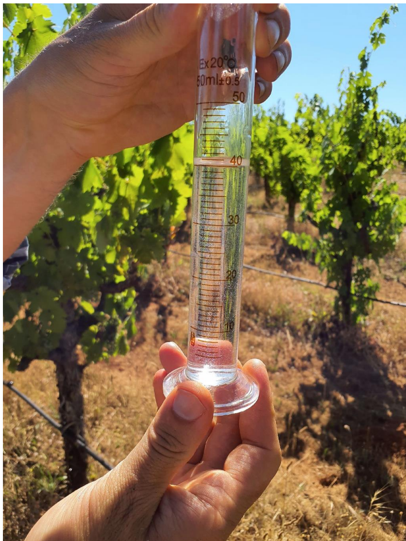
Figure 2-3. Distribution uniformity (DU) testing example, showing the volume measured at a randomly selected drip emitter over a recorded period of time, within a vineyard irrigated by a drip irrigation system.
