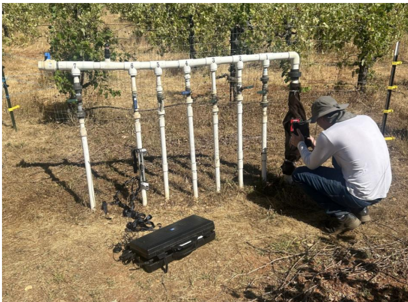
Figure 2-5. Water meter and portable ultrasonic transit time flowmeter measuring the same flow through PVC irrigation pipelines as an evaluation of water meter accuracy. The pipeline furthest right measures all water inflow and includes a permanent water meter; valves can be used to control irrigation to specific blocks on all pipes further to the left. Note that valves on all irrigation blocks except 5 and 6 are closed, and block 5 was closed at another valve further downstream (confirmed in the field), so the flow past the portable meter installed on the block 6 line was equal to the total inflow measured by the permanent water meter.
